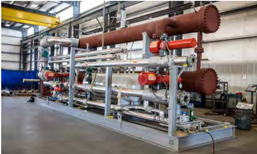
Fuel Gas Performance Heater Skid
